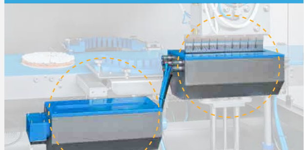
Blades washing and drying automatic system and UV sterilization devices
